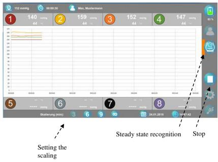
When the automatically calculated steady state value is reached (this can also be skipped manually by pressing the "Steady state recognition" symbol), an acoustic signal sounds and it is represented visually by a line.
